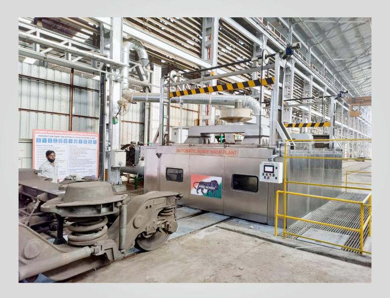
We offer Complete Bogie cleaning plant (Rail feed Type) for Locomotive, Passenger & Transit Car (wagon) Bogies on turnkey basis with complete Automatic process which removes all kinds of exterior contaminations in the bogies that includes primary & secondary coil spring, axle box, wheel sets and all other accessories in the Bogie shop
