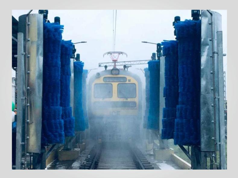
The Automatic Drive through Train Wash Plant automatically clean exterior lateral sides of the rail cars along with the windows.
